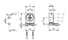
L1-13.6: Recommended dimension - The distance between the cut-outs and the tolerance should be governed by the dimensions of the respective lamps and luminaires.
